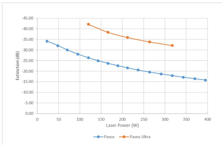
Figure 3: Effect of Laser Power on PAVOS and PAVOS Ultra Extinction
