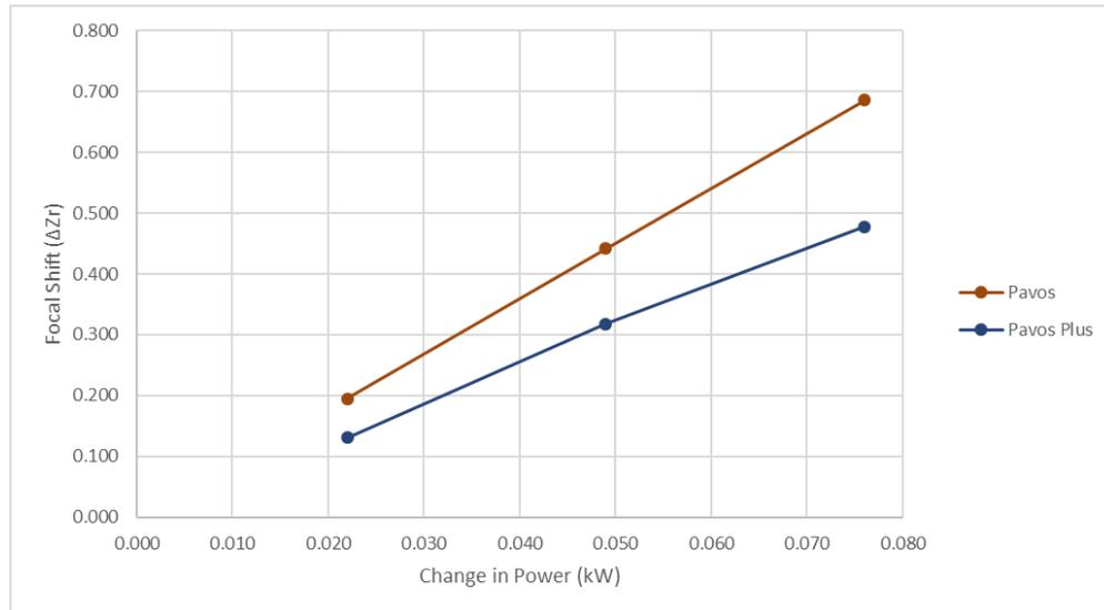
Figure 1: Thermal Lens Focal Shift Comparison
