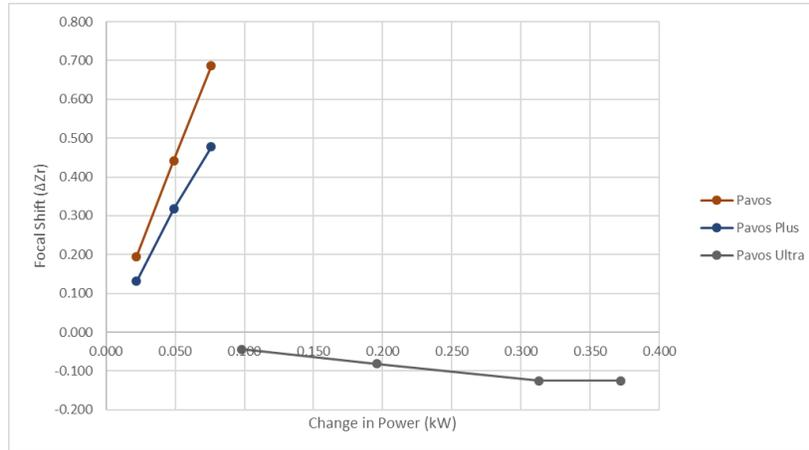
Figure 2: Effect of Laser Power on Focal Shift
